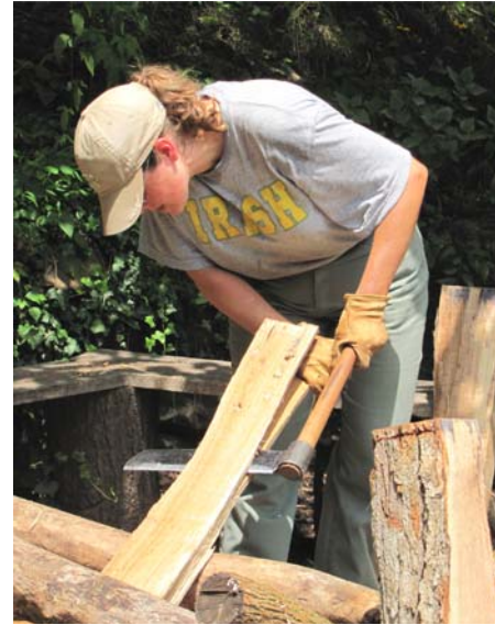
(Left) Wayna Adams, a preservation student, uses a froe to split rough shingles. (Right) Three generations of the Creech family – Bethanny, Bonnie and Daniel Harmon – use draw knives to shape shingles.
