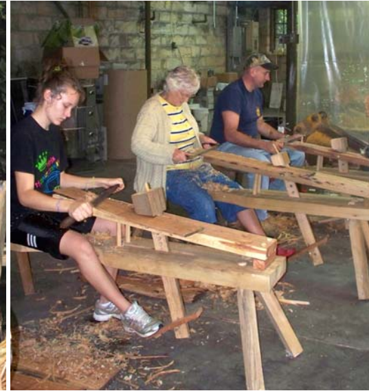
(Left) Wayna Adams, a preservation student, uses a froe to split rough shingles. (Right) Three generations of the Creech family – Bethanny, Bonnie and Daniel Harmon – use draw knives to shape shingles.
